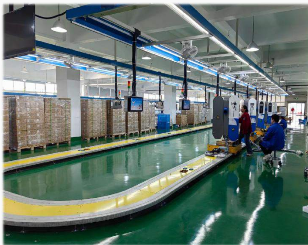
RGV (rail guide vehicle) With SOP (Standard Operating Procedure) Display
